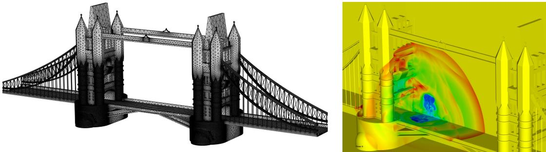
Figure 3.20 – Tower-bridge test case. Initial mesh and geometry (left) and density iso-values of the blast on an adapted mesh (right).
